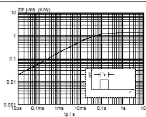
Fig. 11. Transient thermal impedance  $Z_{th,j\text{-mb}}$ , versus pulse width  $t_p$ .
