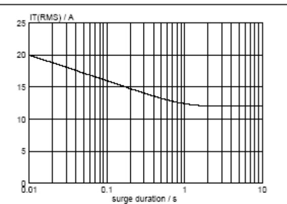
Fig.5. Maximum permissible repetitive rms on-state current  $I_{T(RMS)}$ , versus surge duration, for sinusoidal currents,  $f = 50$  Hz;  $T_{mb} \leq 109^\circ\text{C}$ .
