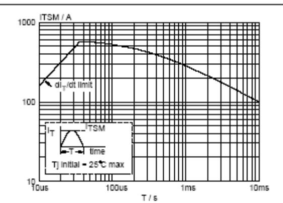
Fig.2. Maximum permissible non-repetitive peak on-state current  $I_{TSM}$ , versus pulse width  $t_p$ , for sinusoidal currents,  $t_p \leq 10$  ms.
