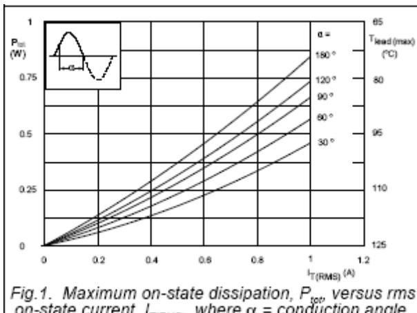
Fig.1. Maximum on-state dissipation,  $P_{oss}$ , versus rms on-state current,  $I_{TRMS}$ , where  $\alpha$  = conduction angle.
