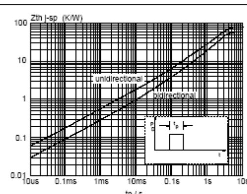
Fig.11. Transient thermal impedance  $Z_{th,I-sp}$  versus pulse width  $t_p$ .
